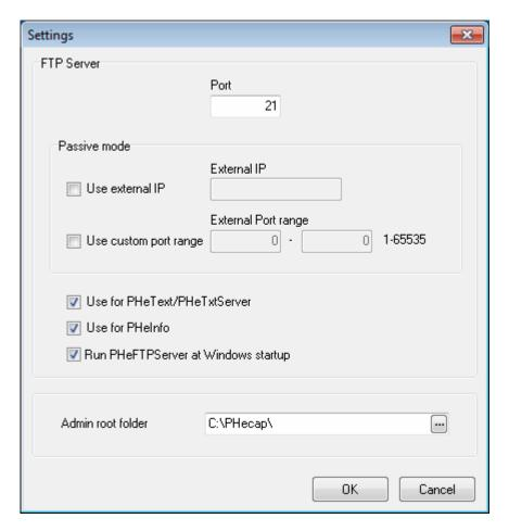
Check "Use PHeText" and/or "Use PHeInfo" if needed. Change the port number when needed. Check "Run PHeFTPServer at Windows startup" if you want to start the program automatically.
