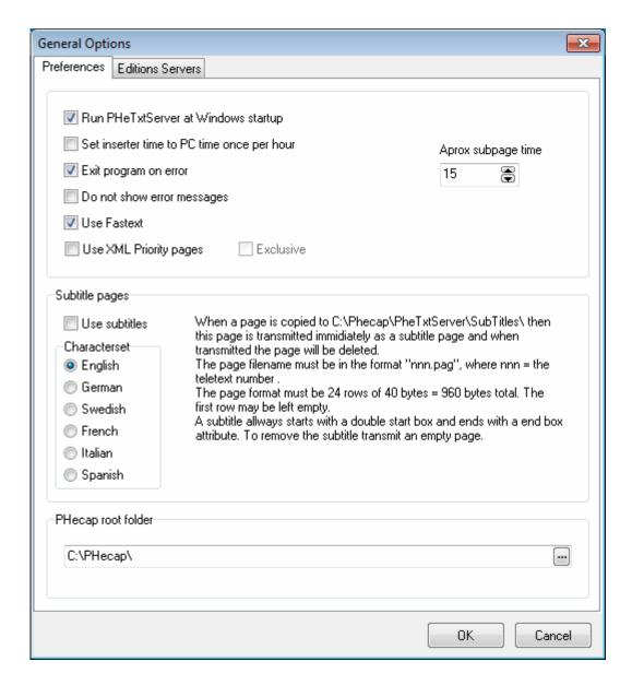
Check "Run PHeTxtServer at Windows startup" if you want to start the program automatically. Check "Use Fastext" if needed.
