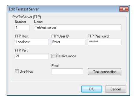
Fill in the FTP Host, UserID and Password. If you use the PHeText program on the same computer as the PHeTxtServer, you can fill in "LocalHost" or 127.0.0.1 as the FTP Host.
